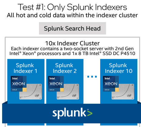
Figure 2. Our first test configuration placed all hot and cold data within the indexer cluster, reflecting a conventional hyperconverged design approach.
